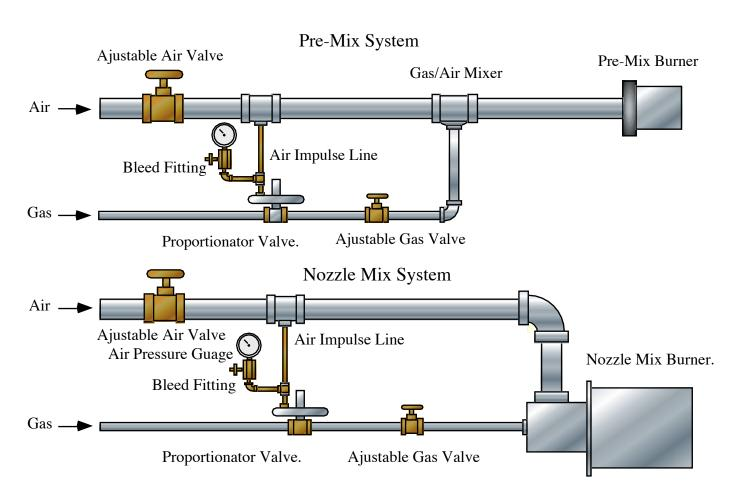
The system is now set up for manual single valve control of the furnace firing range. To turn the furnace up, open the main air valve. To turn it down, close the valve. Now we can install a programmable controller and motorized air valve to control the firing of the furnace.
